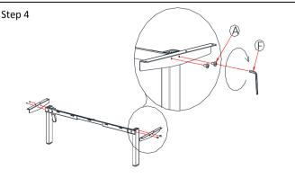
Attach the Side bracket (part 4) to the Crossbeam (part 6) using (part A) Screw M6x10.
