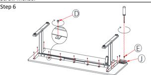
Adjust Crossbeams to the proper position to fit the desktop. Tighten the (part D) Wood screw ST4.8x16 to lock. Attach the Handset (part J) to the underside of the desktop using (part E) Wood screw ST4.2x16.
