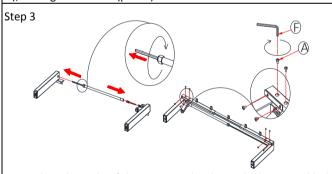
Insert the other side of the Hexagonal rod into the hexagonal hole of the Left lifting leg (part 3) and Right lifting leg (part 2), and attach the Crossbeam (part 6) to the Lifting leg (parts 2 and 3) using (part A) Screw M6x10.
